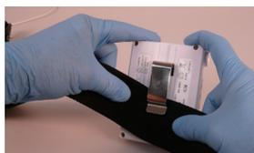
1. Place the top edge of the Belt under the Battery Clip. Move the Belt fully under and up to the top of the Clip.
