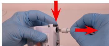
1. Disconnect the Helmet Power Cord from the Battery - push the Secure Connection Button down, pull Cord Connector out, release the Button.
