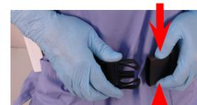
2. Press together the release tabs on the female buckle, disconnect the buckle, then remove the battery and belt from around the waist.
