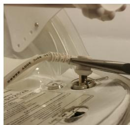
2. Firmly lift the Power Cord-to-Helmet Connector up and out of the Helmet receptacle.
