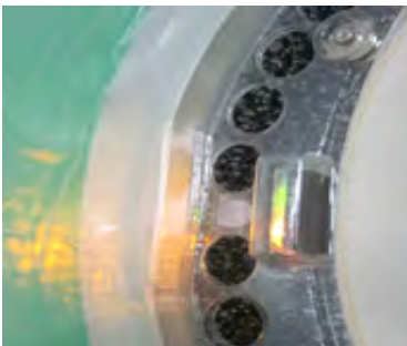
3. Allow the Helmet to compensate until the Yellow LED turns on (about 45 seconds with Air Flow set to High, about 90 seconds with Air Flow set to Low).
